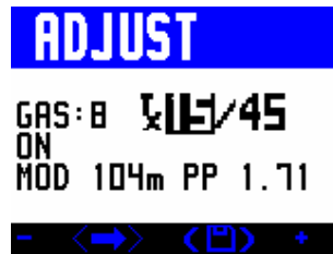
ADJUST screen Trimix O2% highlighted
